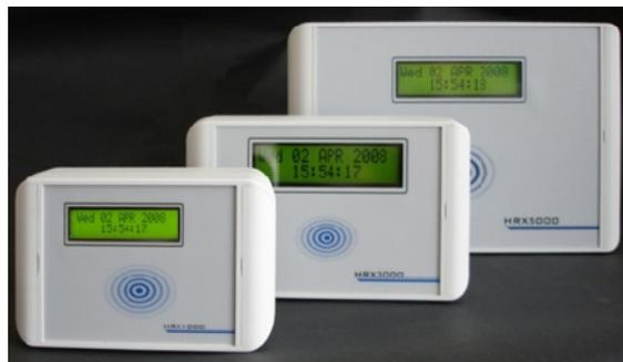
The HRX terminal series are specifically designed to operate with the Focus Time & Attendance software. They provide a highly reliable means of data collection with a wide range of functionality options.
